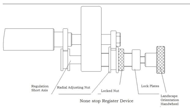
First make rough positioning. Press in the printing cylinder. When the error of the printing trace is around 3.5mm, accurate positioning can be made. However, when the error is greater than 3.5mm, the gear must be withdrawn and turned to the necessary position. Press in the printing cylinder again to make the error around 3.5mm. Switch on
