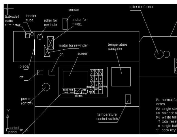
Temperature Control Switch and Temperature Controller use for HOT CUTTING FUNCTION and the blade should be change hot cutting blade
