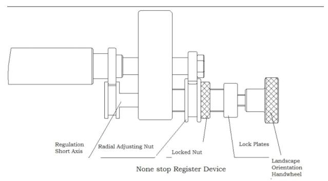
First make rough positioning. Press in the printing cylinder. When the error of the printing trace is around 3.5mm, accurate positioning can be made. However, when the error is greater than 3.5mm, the gear must be withdrawn and turned to the necessary position. Press in the printing cylinder again to make the error around 3.5mm. Switch on
